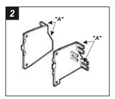
Cut and remove all mounting tabs on **Bracket Set #2** EXCEPT tabs **"A"**. The mounting tabs can be identified by the stamped letter on the back of each tab. Skip to the Installation Instructions for ALL VEHICLES on Page #10.
