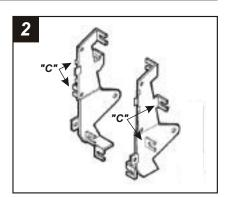
Cut and remove all mounting tabs on **Bracket Set #3** EXCEPT tabs **"C"**. The mounting tabs can be identified by the stamped letter on the back of each tab. Skip to the Installation Instructions for ALL VEHICLES on Page #10.
