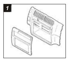
Disconnect the negative battery terminal to prevent an accidental short circuit. Pull the cupholder out and unsnap the trim bezel from the dash. Remove (4) screws securing the factory head unit and disconnect the wiring.
