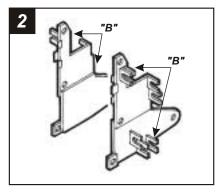
Cut and remove all mounting tabs on **Bracket Set #1** EXCEPT top tabs **"B"**. The mounting tabs can be identified by the stamped letter on the back of each tab. *Skip to the Installation Instruc-tions for ALL VEHICLES on Page #10*.
