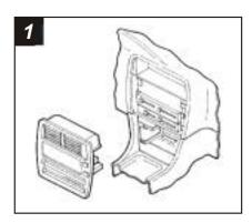
Disconnect the negative battery terminal to prevent an accidental short circuit. Remove the climate control knobs and unsnap the dash trim bezel. Disconnect the clock and hazard leads.
