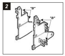
Cut and remove all mounting tabs on **Bracket Set #1** EXCEPT tabs **"B"**. The mounting tabs can be identified by the stamped letter on the back of each tab. *Skip to the Installation Instructions for ALL VEHICLES on Page #10*.
