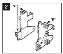
Cut and remove all mounting tabs on **Bracket Set #4** EXCEPT tabs **"B"**. The mounting tabs can be identified by the stamped letter on the back of each tab. Skip to the Installation Instructions for ALL VEHICLES on Page #10.
