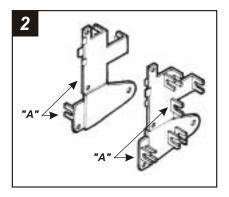
Cut and remove all mounting tabs on **Bracket Set #4** EXCEPT tabs **"A"**. The mounting tabs can be identified by the stamped letter on the back of each tab. **Skip** to the **Installation Instructions** for **ALL VEHICLES** on **Page** #10.
