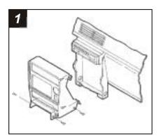
Disconnect the negative battery terminal to prevent an accidental short circuit. Remove (2) screws from the lower steering column panel and remove. Remove the (2) screws exposed on the radio trim bezel. Open the glove box and remove (1) screw and (1) bolt exposed. Remove (2) screws from the ashtray cavity and (2) screws from the bracket. Remove (2) screws from each lower side of the trim bezel and unsnap the bezel.
