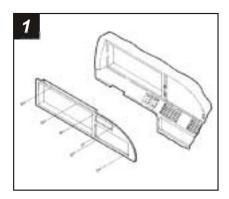
Disconnect the negative battery terminal to prevent an accidental short circuit. Remove (4) screws from the top edge of the instrument trim bezel and (2) screws below the radio opening. Remove (1) screw from the lower-left tab of the bezel ( to the right of the a/c vent) and unsnap the bezel.
