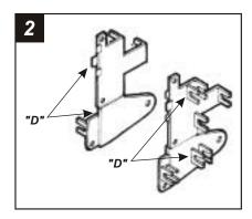
Cut and remove all mounting tabs on *Bracket Set #4* EXCEPT tabs "D". The mounting tabs can be identified by the stamped letter on the back of each tab. *Skip to the Installation Instructions for ALL VEHICLES on Page #10.*
