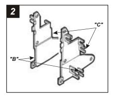
Cut and remove all mounting tabs on **Bracket Set #1** EXCEPT top tabs **"C"** and bottom tabs **"B"**. The mounting tabs can be identified by the stamped letter on the back of each tab. Skip to the Installation Instructions for ALL VEHICLES on Page #10.
