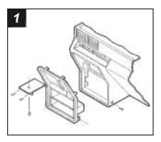
Disconnect the negative battery terminal to prevent an accidental short circuit. Remove the ashtray and (3) screws from the ashtray bracket. Remove (1) screw from each side of the dash console and unsnap the trim bezel.
