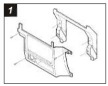
Disconnect the negative battery terminal to prevent an accidental short circuit. Remove the driver's side speaker panel by removing (3) screws and (1) 10mm bolt. Remove (1) screw from the left side of the housing and unsnap the ignition cover. Remove the glove compartment assembly by removing (1) 10mm bolt from the bottom of the speaker panel and (3) screws from the right side of the housing. Remove the remaining (3) screws securing the radio trim bezel.
