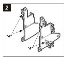
Cut and remove all mounting tabs on **Bracket Set #1** EXCEPT tabs **"A"**. The mounting tabs can be identified by the stamped letter on the back of each tab. Skip to the Installation Instructions for ALL VEHICLES on Page #10.
