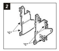
Cut and remove all mounting tabs on **Bracket Set #1** EXCEPT tabs **"C"**. The mounting tabs can be identified by the stamped letter on the back of each tab. Skip to the Installation Instructions for ALL VEHICLES on Page #10.
