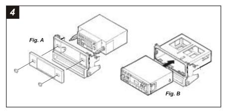
**2-SHAFT HEAD UNITS:** Attach the **Faceplate** to the **Radio Housing**. Slide the aftermarket head unit into the kit and secure with shaft nuts. (see Fig. A)
