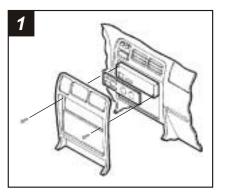
Disconnect the negative battery terminal to prevent an accidental short circuit. Open the center armrest door. Unsnap the parking brake trim panel to access the gear shifter trim panel. Unsnap the gear shifter trim panel and remove. Remove the climate control knobs. Remove the climate control trim plate and (2) Phillips screws exposed. Unclip the radio trim bezel and remove. Remove (4) Phillips screws securing the factory head unit and disconnect the wiring.
