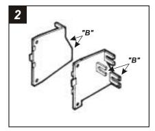
Cut and remove all mounting tabs on *Bracket Set #2* EXCEPT tabs "B". The mounting tabs can be identified by the stamped letter on the back of each tab. *Skip to the Installation Instructions for ALL VEHICLES on Page #10.*
