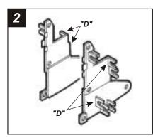
Cut and remove all mounting tabs on **Bracket Set #1** EXCEPT tabs **"D"**. The mounting tabs can be identified by the stamped letter on the back of each tab. **Skip** to the Installation Instructions for ALL **VEHICLES** on Page #10.
