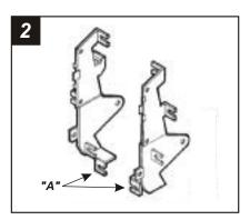
Cut and remove all mounting tabs on **Bracket Set #3** EXCEPT tabs **"A"**. The mounting tabs can be identified by the stamped letter on the back of each tab. **Skip** to the Installation Instructions for ALL VEHICLES on Page #10.
