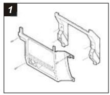
Disconnect the negative battery terminal to prevent an accidental short circuit. Remove the driver's side speaker panel by removing (3) screws and (1) 10mm bolt. Remove (1) screw from the left side of the housing and unsnap the ignition cover. Remove the glove compartment assembly by removing (1) 10mm bolt from the bottom of the speaker panel and (3) screws from the right side of the housing. Remove the remaining (3) screws securing the radio trim bezel.
