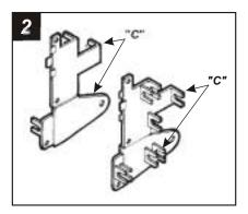
Cut and remove all mounting tabs on **Bracket Set #4** EXCEPT tabs **"C"**. The mounting tabs can be identified by the stamped letter on the back of each tab. Skip to the Installation Instructions for ALL VEHICLES on Page #10.
