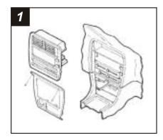
Disconnect the negative battery terminal to prevent an accidental short circuit. Remove the climate control knobs, unsnap the upper trim bezel and disconnect the hazard and clock leads. Remove (2) screws from the lower trim bezel and remove.
