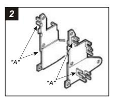
Cut and remove all mounting tabs on **Bracket Set #1** EXCEPT tabs **"A"**. The mounting tabs can be identified by the stamped letter on the back of each tab. Skip to the Installation Instructions for ALL VEHICLES on Page #10.
