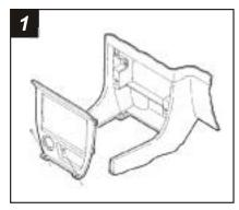
Disconnect the negative battery terminal to prevent an accidental short circuit. Carefully pry up on the gear shifter trim panel and remove. Remove (2) screws exposed on the bottom edge of the radio trim panel. Unsnap the panel and disconnect the ashtray and cigarette lighter wiring.
