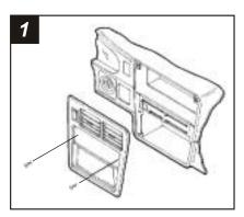
Disconnect the negative battery terminal to prevent an accidental short circuit. Remove the climate control knobs. Unsnap the climate control trim panel and remove (2) screws exposed. Gently unclip the dash trim bezel, lift up on the panel and remove.
