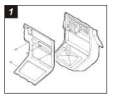
Disconnect the negative battery terminal to prevent an accidental short circuit. Remove the ashtray and (2) screws from the ashtray cavity. Remove (1) screw located to the right of the steering column, and (1) screw located to the left of the gear shifter.
