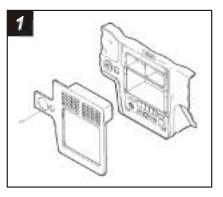
Disconnect the negative battery terminal to prevent an accidental short circuit. Remove the ashtray and (2) screws from the ashtray cavity. Unsnap and remove the shifter console bezel. Remove (1) screw below the ignition switch and remove the dash trim bezel.
