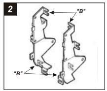
Cut and remove all mounting tabs on **Bracket Set #3** EXCEPT tabs **"B"**. The mounting tabs can be identified by the stamped letter on the back of each tab. Skip to the Installation Instructions for ALL VEHICLES on Page #10.
