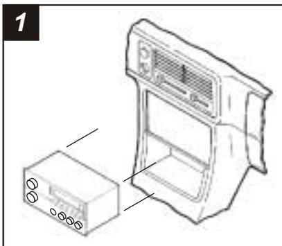
Disconnect the negative battery terminal to prevent an accidental short circuit. Remove (3) screws from each side of the center console and remove the console. Remove (2) screws securing the factory head unit to the sub-dash support bracket. Slide the head unit/pocket assembly out and disconnect the wiring.
