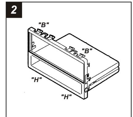
Cut and remove the all mounting clips on the **Radio Housing** EXCEPT clips "B" and "H". (The clips can be identified by the stamped letter near each clip). Skip to step #3b on Page 11.
