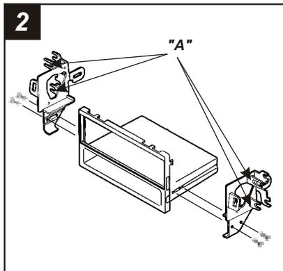
Cut and remove the mounting clips from the **Radio Housing**. Locate tabs "A" on the **Mounting Brackets** for mounting, cut and remove tabs "B". (The tabs can be identified by the stamped letter near each tab). Secure the Brackets to the Housing with (4) #8 x 3/8" Phillips Pan-head Screws. Skip to step #3b on Page 11.
