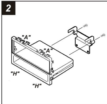
Cut and remove the all mounting clips on the **Radio Housing** EXCEPT clips "A" and "H". (The clips can be identified by the stamped letter near each clip). Mount the **Rear Support Bracket #R1** to the back of the Radio Housing with (2) #8 x 3/8" Phillips Pan-head Screws supplied. Skip to step #3b on Page 11.
