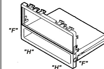
Cut and remove the all mounting clips on the **Radio Housing** EXCEPT clips "F" and "H". (The clips can be identified by the stamped letter near each clip). Skip to step #3b on Page 11.
