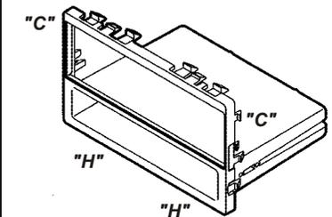
Cut and remove the all mounting clips on the **Radio Housing** EXCEPT clips "C" and "H". (The clips can be identified by the stamped letter near each clip). Skip to step #3b on Page 11.
