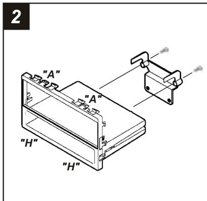
Cut and remove the all mounting clips on the **Radio Housing** EXCEPT clips "A" and "H". (The clips can be identified by the stamped letter near each clip). Mount the **Rear Support Bracket #R1** to the back of the Radio Housing with (2) #8 x 3/8" Phillips Pan-head Screws supplied. Skip to step #3b on Page 11.
