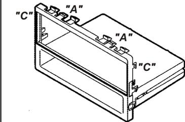
Cut and remove the all mounting clips on the **Radio Housing** EXCEPT clips "A" and "C". (The clips can be identified by the stamped letter near each clip). Skip to step #3b on Page 11.
