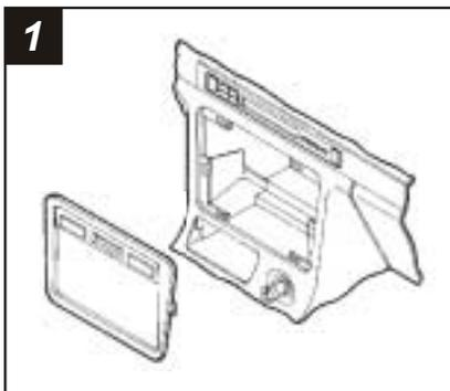
Disconnect the negative battery terminal to prevent an accidental short circuit. Unclip the radio trim bezel and disconnect the clock and climate control wiring. Remove (2) 8mm hex-head screws securing the factory head unit and disconnect the wiring.
