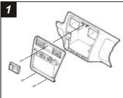
Disconnect the negative battery terminal to prevent an accidental short circuit. Unsnap the clock panel, disconnect the wiring and remove. Remove (1) Phillips screw exposed in the clock cavity. Remove (2) Phillips screws below the factory head unit. Unclip the radio trim bezel and disconnect the wiring. Remove (4) Phillips screws securing the factory head unit assembly and disconnect the wiring. Remove (2) screws securing the factory pocket to the assembly.
