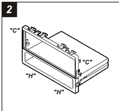
Cut and remove the all mounting clips on the **Radio Housing** EXCEPT clips "C" and "H". (The clips can be identified by the stamped letter near each clip). Skip to step #3b on Page 11.
