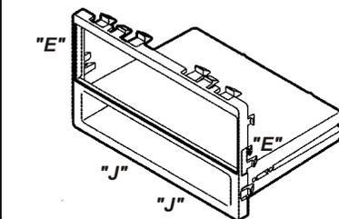
Cut and remove the all mounting clips on the **Radio Housing** EXCEPT clips "E" and "J". (The clips can be identified by the stamped letter near each clip). Skip to step #3b on Page 11.
