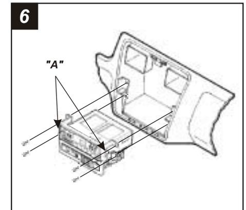
Re-connect the battery terminal and test the unit for proper operation. Mount the head unit/kit assembly to the sub-dash with (4) Phillips screws previously removed in step #1. Re-attach the radio trim bezel. Be sure the clips on the back of the bezel engage slots "A" on the kit.
