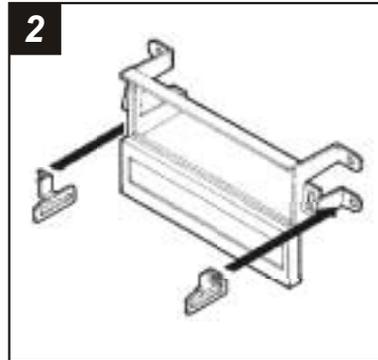
Snap the **Brackets** onto the front of the lower mounting tabs on the **Radio Housing**.
