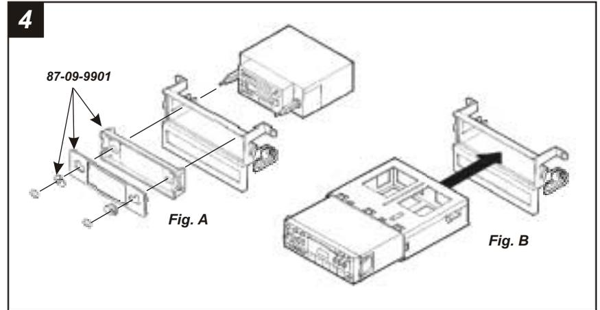
**2-SHAFT HEAD UNITS:** Order Metra's **87-09-9901** and snap it into the **Radio Housing**. Slide the aftermarket unit into the kit and secure with shaft nuts. (see Fig. A)
