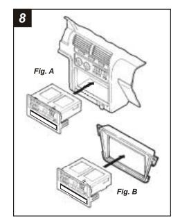
INTEGRA, ACCORD, ODYSSEY, OASIS: Reconnect the battery terminal and test the unit for proper operation. Snap the head unit/kit assembly into the sub-dash. (see Fig. A)
