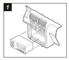
Disconnect the negative battery terminal to prevent an accidental short circuit. Remove (4) screws from the lower portion of the center console. Remove the gear shifter knob and lift the console out. Remove the ashtray and ashtray bracket. Remove (2) screws from the bottom of the head unit support, slide the unit out and disconnect the wiring.
