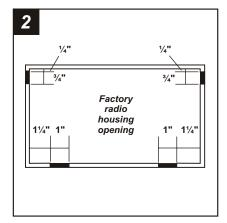
Modify the factory radio housing by cutting and removing the *shaded* portions of the housing lip. *Skip to the Installation Instructions for ALL VEHICLES on Page #5.*
