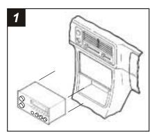
Disconnect the negative battery terminal to prevent an accidental short circuit. Remove (3) screws from each side of the center console and remove the console. Remove (2) screws securing the factory head unit to the sub-dash support bracket. Slide the head unit/pocket assembly out and disconnect the wiring.
