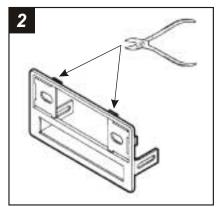
Cut and remove the *TOP* clips from the *Radio Housing*. Skip to the Installation Instructions for ALL VEHICLES on Page #5.
