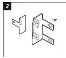
Locate **Bracket #(L) S-10** and the right Bracket from **Bracket Set #5.** Cut and remove all mounting tabs on the right Bracket EXCEPT top tab "B". The mounting tabs can be identified by the stamped letter on the back of each tab. Skip to the Installation Instructions for ALL VEHICLES on Page #34.
