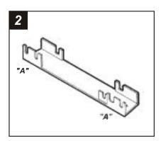
Cut and remove all mounting tabs on **Bracket #6** EXCEPT tabs **"A"**. The mounting tabs can be identified by the stamped letter on the back of each tab. **Skip** to the Installation Instructions for ALL VEHICLES on Page #34.
