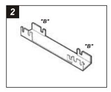
Cut and remove all mounting tabs on **Bracket #6** EXCEPT tabs **"B"**. The mounting tabs can be identified by the stamped letter on the back of each tab. Skip to the Installation Instructions for ALL VEHICLES on Page #34.
