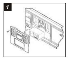
Disconnect the negative battery terminal to prevent an accidental short circuit. Remove (2) Phillips screws above the a/c vents. Pull out on the top edge of the dash trim bezel unhook the bottom edge and remove.
