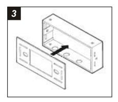
Choose a Faceplate (according to the desired installation depth) and snap it onto the front of the Radio Housing. (If an equalizer will be included in the installation, the **Equalizer Faceplate** must be used).
