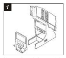
Disconnect the negative battery terminal to prevent an accidental short circuit. Unsnap the gear shifter bezel from the base of the console. Remove (2) screws securing the bottom of the dash trim bezel and remove the bezel.
