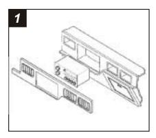
Disconnect the negative battery terminal to prevent an accidental short circuit. Remove (2) screws from the lower steering column panel. Pull the panel down to access the bottom portion of the radio trim bezel. Pull the top and bottom edges of the bezel forward and remove.
