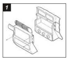
Disconnect the negative battery terminal to prevent an accidental short circuit. Remove (6) 7mm hex-head screws from the driver's side knee bolster panel and lower the panel. Remove (4) Phillips screws from the glove box/cupholder assembly. Remove (1) 7mm hex-head screw from the left corner of the dash trim bezel. Loosen (2) 10mm nuts from the top of the factory head unit, slide the unit out and disconnect the wiring.
