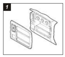
Disconnect the negative battery terminal to prevent an accidental short circuit. Unclip the plastic trim piece located below the steering column. Unclip the dash trim bezel. Pull the bezel over the steering column and disconnect the wiring. Using a flat-blade screwdriver, press down on the outside clips of the factory head unit and remove. Skip to the Installation Instructions for ALL VEHICLES on Page #2.
