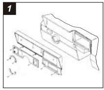
Disconnect the negative battery terminal to prevent an accidental short circuit. Remove the ashtray and (2) screws from the ashtray location. Remove (1) screw below and (2) screws above the steering column. Pry the a/c vents out and remove the screws exposed in the vent cavities. Remove (6) screws from the edge of the dash trim bezel and remove the bezel
