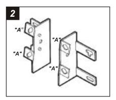
Cut and remove all mounting tabs on **Bracket #5** EXCEPT tabs **"A"**. The mounting tabs can be identified by the stamped letter on the back of each tab. Skip to the Installation Instructions for ALL VEHICLES on Page #34.
