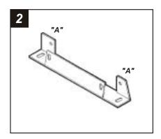
Cut and remove all mounting tabs on **Bracket #4** EXCEPT tabs **"A"**. The mounting tabs can be identified by the stamped letter on the back of each tab. **Skip** to the Installation Instructions for ALL **VEHICLES** on Page #34.
