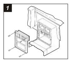
Disconnect the negative battery terminal to prevent an accidental short circuit. Remove (4) star-drive screws from the dash trim bezel. Gently pull out on the trim bezel and remove. Remove (4) hex-head screws from the factory head unit and disconnect the wiring.
