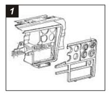
Disconnect the negative battery terminal to prevent an accidental short circuit. Remove (3) screws from the top edge of the dash trimbezel. Remove (4) screws from the metal steering column trim and remove the trim. Remove (4) screws exposed at the bottom edge of the dash trim bezel. Remove the cigarette lighter and retainer ring and remove the dash trim bezel.
