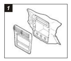
Disconnect the negative battery terminal to prevent an accidental short circuit. Unclip the radio trim bezel and remove. Remove (2) 7mm hex-head screws securing the factory head unit and disconnect the wiring.
