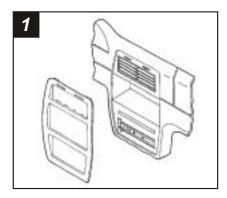
Disconnect the negative battery terminal to prevent an accidental short circuit. Gently unclip the dash trim bezel. Remove (2) screws from the factory head unit and disconnect the wiring.
