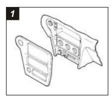
Disconnect the negative battery terminal to prevent an accidental short circuit. Remove the ashtray and (1) Phillips screw exposed in the ashtray cavity. Remove (1) Phillips screw from the cigarette lighter compartment. Remove (2) Phillips screws securing the factory head unit and disconnect the wiring.
