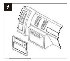
Disconnect the negative battery terminal to prevent an accidental short circuit. Remove the radio knobs and cigarette lighter. Gently unclip the radio trim bezel and remove.
