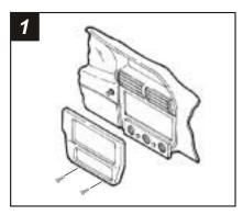
Disconnect the negative battery terminal to prevent an accidental short circuit. Using a small set of pliers, grasp the retaining clip on the back of the gear shifter handle and remove the clip. Remove the gear shifter handle. Unclip the center console and remove. Remove (2) 7mm hex-head screws exposed under the climate controls. Unclip the radio trim bezel and remove. Remove (2) 7mm hex-head screws securing the factory head unit and disconnect the wiring.
