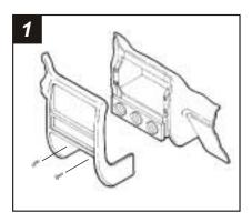
Disconnect the negative battery terminal to prevent an accidental short circuit. Remove (2) Phillips screws from the pocket. Remove (2) Phillips screws above the instrument cluster. Unclip the dash trim bezel and remove. Remove (3) 7mm hex-head screws securing the factory head unit and disconnect the wiring.
