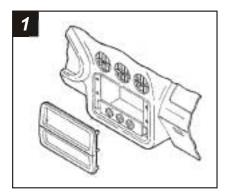
Disconnect the negative battery terminal to prevent an accidental short circuit. Unclip the radio trim bezel. Remove (4) 7mm hexhead screws securing the factory head unit and disconnect the wiring.
