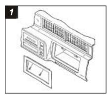
Disconnect the negative battery terminal to prevent an accidental short circuit. Remove (2) screws from the top of the radio trim bezel. Pull out on the top edge of the bezel and lift up to remove.
