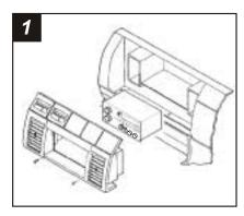
Disconnect the negative battery terminal to prevent an accidental short circuit. Remove (2) screws from the bottom of the dash trim bezel. Gently unclip and remove the bezel. Remove (4) screws from the factory head unit and disconnect the wiring.
