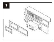
Disconnect the negative battery terminal to prevent an accidental short circuit. Unsnap the climate control trim bezel and remove (4) star-drive screws exposed. Pull the steering collar back and carefully unsnap the dash trim bezel.
