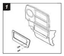
Disconnect the negative battery terminal to prevent an accidental short circuit. Remove (2) screws from the radio trim bezel and remove the bezel. Remove (2) screws securing the factory head unit and disconnect the wiring.
