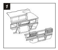
Disconnect the negative battery terminal to prevent an accidental short circuit. Place the gear shifter in low and remove the rubber trim boot from the steering column. Remove (2) Phillips screws from the radio trim bezel. Unhook the ashtray/light wiring terminal and remove the trim bezel.
