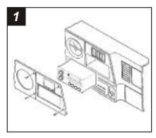
Disconnect the negative battery terminal to prevent an accidental short circuit. Remove (6) star-drive screws from the dash trim bezel and remove the bezel. Remove (2) screws from the factory head unit and disconnect the wiring.
