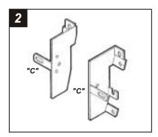
Cut and remove all mounting tabs on **Bracket #1** EXCEPT tabs **"C"**. The mounting tabs can be identified by the stamped letter on the back of each tab. **Skip** to the Installation Instructions for ALL VEHICLES on Page #34.
