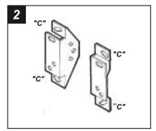
Cut and remove all mounting tabs on **Bracket #2** EXCEPT tabs **"C"**. The mounting tabs can be identified by the stamped letter on the back of each tab. **Skip** to the Installation Instructions for ALL **VEHICLES** on Page #34.
