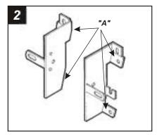
Cut and remove all mounting tabs on **Bracket #1** EXCEPT tabs **"A"**. The mounting tabs can be identified by the stamped letter on the back of each tab. **Skip** to the Installation Instructions for ALL VEHICLES on Page #34.
