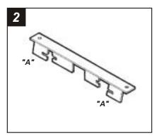
Cut and remove all mounting tabs on **Bracket #3** EXCEPT tabs **"A"**. The mounting tabs can be identified by the stamped letter on the back of each tab. Skip to the Installation Instructions for ALL VEHICLES on Page #34.
