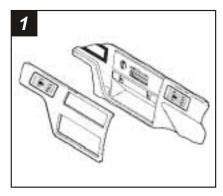
Disconnect the negative battery terminal to prevent an accidental short circuit. Gently unsnap and remove the dash trim bezel. Remove the screws securing the factory head unit and disconnect the wiring.
