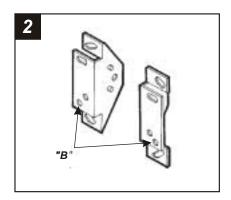
Cut and remove all mounting tabs on **Bracket #2** EXCEPT those tabs with holes **"B"**. The mounting tabs can be identified by the stamped letter on the back of each tab. Skip to the Installation Instructions for ALL VEHICLES on Page #34.
