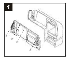
Disconnect the negative battery terminal to prevent an accidental short circuit. Remove (2) torx-head screws above the instrument cluster and (1) torx-head screw from each a/c vent. Unsnap the panel.
