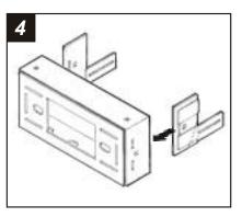
Slide the Equalizer Brackets into the slots along the inner walls of the Radio Housing.
