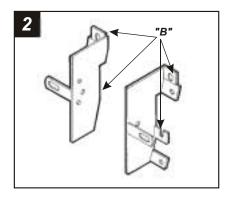
Cut and remove all mounting tabs on **Bracket #1** EXCEPT tabs **"B"**. The mounting tabs can be identified by the stamped letter on the back of each tab. Skip to the Installation Instructions for ALL VEHICLES on Page #34.
