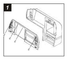
Disconnect the negative battery terminal to prevent an accidental short circuit. Remove (2) torx-head screws above the instrument panel. Remove (1) torx-head screw from each a/c vent. Unclip the dash trim bezel and remove.
