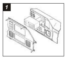
Disconnect the negative battery terminal to prevent an accidental short circuit. Remove (2) screws from the driver's side service panel and unclip the panel. Pry off the trim piece located above the glove box and remove (1) screw. Remove (3) screws from the top edge of the dash trim bezel. Remove (1) screw from the lower-left corner of the glove box and (1) screw from the parking brake release. Remove the dash trim bezel.
