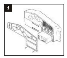
Disconnect the negative battery terminal to prevent an accidental short circuit. Remove (4) screws from the top edge of the dash trim bezel. Remove (2) screws from the bottom edge of the bezel. Unsnap the a/c ducts, disconnect the light switch and remove the bezel.
