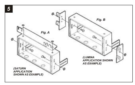
TOP AND/OR BOTTOM MOUNTING BRACKETS: Mount the Equalizer Brackets to the Radio Housing with (2) Carriage Bolts and (2) Keps Nuts. Secure the Mounting Bracket(s) to the Housing with Carriage Bolts and Keps Nuts. (see Fig. A)
