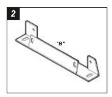
Cut and remove all mounting tabs on **Bracket #4** EXCEPT tabs **"B"**. The mounting tabs can be identified by the stamped letter on the back of each tab. **Skip** to the Installation Instructions for ALL VEHICLES on Page #34.
