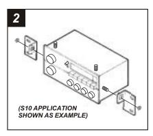
Remove the hardware securing the factory mounting brackets to the factory head unit. Remove and retain the brackets. Skip to the Installation Instructions for ALL VEHICLES on Page #34.
