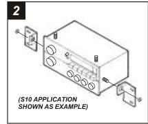
Remove the hardware securing the factory mounting brackets to the factory head unit. Remove and retain the brackets. Skip to the Installation Instructions for ALL VEHICLES on Page #34.
