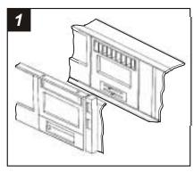
Disconnect the negative battery terminal to prevent an accidental short circuit. Remove (4) screws from the top-inside edge of the dash trim bezel. Remove (5) screws from both sides of the steering column. Remove (3) Phillips screws securing the rockerswitch housing and lift the housing out. Remove the bezel.
