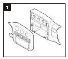
Disconnect the negative battery terminal to prevent an accidental short circuit. Unclip the dash trim bezel and remove. (It may be necessary to loosen the knee bolster). Remove (2) 7mm hex-head screws securing the factory head unit and disconnect the wiring.
