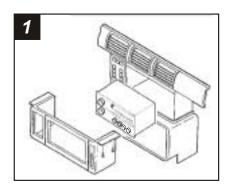
Disconnect the negative battery terminal to prevent an accidental short circuit. Remove (1) Phillips screw from each side of the center console. Open the glove box and remove (2) Phillips screws exposed. Remove (2) 7mm hex-head screws and (1) pop-clip from the lower steering column panel, and (2) Phillips screws exposed near the climate controls. Remove (1) 7mm hex-head screw under the glove box. Pull out on the center console and remove.
