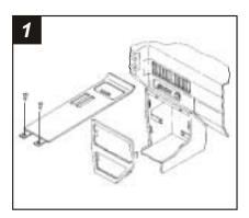
Disconnect the negative battery terminal to prevent an accidental short circuit. Remove the console/glove box assembly and (3) screws below the box. Lift up the parking brake trim and remove (2) screws from the gear shifter trim. Remove the ashtray from the gear shifter area and (2) 7mm screws exposed. Using a screwdriver, depress the retainer tabs on the dash ashtray, pull the ashtray out and remove (2) 7mm hex-head screws from the ashtray bracket.
