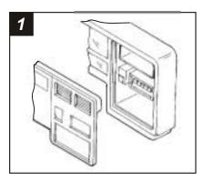
Disconnect the negative battery terminal to prevent an accidental short circuit. Pull out on the ashtray and remove (2) screws exposed in the ashtray cavity. Remove (2) screws securing the front of the ashtray and lower section of the dash trim bezel. Using a panel removal tool, gently pry out on the trim bezel and remove. Remove (2) nuts from the bottom of the factory head unit and disconnect the wiring.
