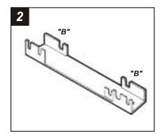
Cut and remove all mounting tabs on **Bracket #6** EXCEPT tabs **"B"**. The mounting tabs can be identified by the stamped letter on the back of each tab. Skip to the Installation Instructions for ALL VEHICLES on Page #34.
