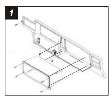
Disconnect the negative battery terminal to prevent an accidental short circuit. Remove the glove box by removing the doorstrap wire clip and (4) screws. Remove (2) screws below the cigarette lighter housing and (3) screws below the steering column. Remove (1) screw from the top-left of the factory head unit and unclip the dash trim bezel.
