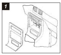
Disconnect the negative battery terminal to prevent an accidental short circuit. Carefully unsnap the front edge of the gear shifter console panel. Unsnap and remove the dash trim bezel.
