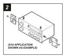
Remove the hardware securing the factory mounting brackets to the factory head unit. Remove and retain the brackets. *Skip to the Installation Instructions for ALL VEHICLES on Page #34.*
