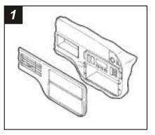
Disconnect the negative battery terminal to prevent an accidental short circuit. Unclip the right side of the dash trim bezel. Unclip the left side of the bezel and remove. Remove (3) 7mm hex-head screws securing the factory head unit and disconnect the wiring.
