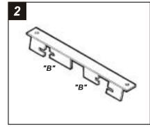
Cut and remove all mounting tabs on **Bracket #3** EXCEPT tabs **"B"**. The mounting tabs can be identified by the stamped letter on the back of each tab. Skip to the Installation Instructions for ALL VEHICLES on Page #34.
