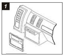
Disconnect the negative battery terminal to prevent an accidental short circuit. Remove the cigarette lighter and radio knobs and unsnap the radio trim bezel. Remove (1) screw from the right side of the ashtray housing.
