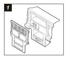
Disconnect the negative battery terminal to prevent an accidental short circuit. Remove (7) screws from the dash trim bezel. Move the gear shifter to the lowest position. Pull the right edge of the bezel forward, unhook the left side and remove.
