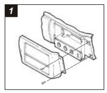
Disconnect the negative battery terminal to prevent an accidental short circuit. Open the glove box and remove (2) Phillips screws exposed on the right edge of the radio trim bezel. Unclip the bezel and remove. Remove (2) 7mm hex-head screws securing the factory head unit and disconnect the wiring.
