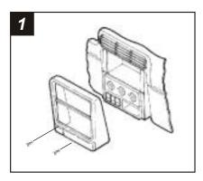
Disconnect the negative battery terminal to prevent an accidental short circuit. Unclip the radio trim bezel and remove. Remove (2) 9/32" hex-head screws securing the factory head unit and disconnect the wiring.
