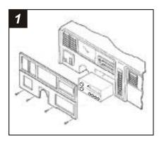
Disconnect the negative battery terminal to prevent an accidental short circuit. Depress the clip located behind the headlight knob and remove the knob. Remove (3) screws securing the steering column trim and remove. Remove (4) screws from the bottom edge of the dash trim bezel and remove.
