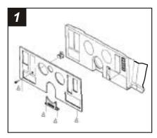
Disconnect the negative battery terminal to prevent an accidental short circuit. Remove (4) screws from the top edge of the instrument panel. Remove (1) screw from the bottom-left corner of the panel. Remove (2) screws from the steering column trim and remove the trim. Pull up and out on the dash trim bezel and remove.
