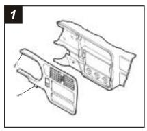
Disconnect the negative battery terminal to prevent an accidental short circuit. Remove (2) 9/32" hex-head screws from the knee bolster. Pull down on the bolster and remove 9/32" screws exposed on the base of the dash trim bezel. Remove (1) Philips screw above the instrument cluster. Unclip the dash trim bezel and remove. Remove (2) 9/32" hex-head screws securing the factory head unit and disconnect the wiring. Skip to the Installation Instructions for ALL VEHICLES on Page #3.
