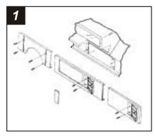
Disconnect the negative battery terminal to prevent an accidental short circuit. Remove the plastic plate next to each a/c vent and remove (2) screws exposed. Remove (4) screws surrounding the steering column. Depress the light control knob spring, remove the knob and lift the bezel off.
