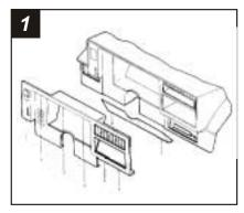
Disconnect the negative battery terminal to prevent an accidental short circuit. Remove (2) screws from the bottom steering column trim panel and remove. Remove (6) screws from the dash trim bezel, disconnect the wiring andremove.
