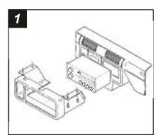
Disconnect the negative battery terminal to prevent an accidental short circuit. Remove (1) 9/32" hex-head screw from the computer diagnostic plug and twist to access (1) 9/32" screw on the trim panel. Remove (3) 9/32" screws from the bottom edge of the panel and remove. Open the glove box and remove (4) 9/32" screws from the dash trim bezel.
