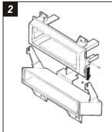
Remove the pocket from the factory head unit and slide the side tabs on the **Radio Housing** between the mounting tabs on the pocket.
