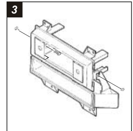
Mount the pocket to the **Radio Housing** with (2) **Carriage Bolts** and (2) **Nuts** supplied.
