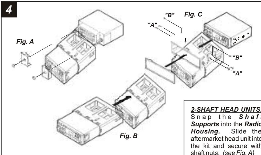
**DIN HEAD UNITS:** Slide the DIN cage into the kit and secure by bending the metal locking tabs down. Slide the aftermarket head unit into the cage until secure. (see Fig. B)
