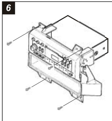
Re-connect the battery terminal and test the unit for proper operation. Mount the head unit/kit assembly to the sub-dash with (4) screws previously removed in step #1.
